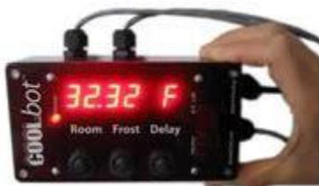
Figure 1: The CoolBot™ controller (Photo source: <http://storeitcold.com>)
