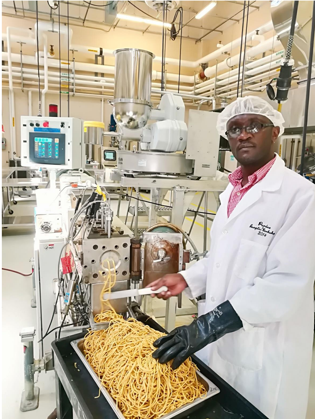
Twin screw extruder
