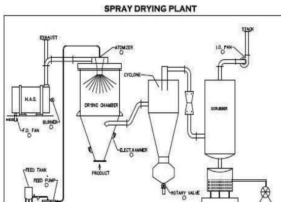
The main components of the drier were the feed system, air compressor with blower, rotary disk atomizer, cyclone and peristaltic pump. The feed system of drying air constituted of a blower and an air filter. The inlet and outlet air temperature were controlled, manually adjusted and the product was collected in a cyclone.
