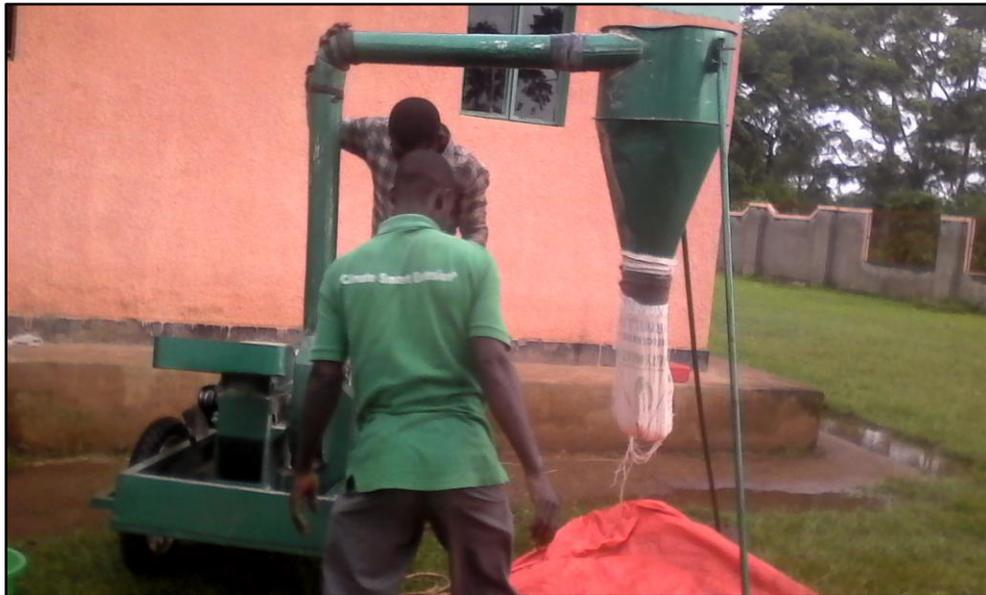
**Figure 7:** Processors milling dried cassava chips using a movable hammer mill.
