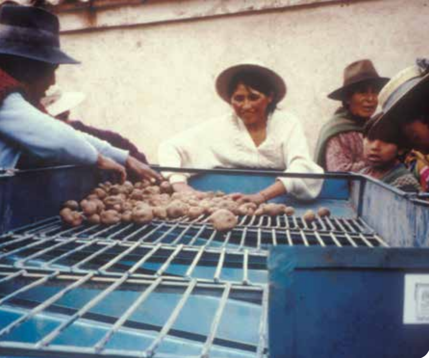
Diverging potato sorter in Bolivia: smaller potatoes drop in between the narrow poles at the base, and larger potatoes make it to the widest - FAO/Katia Iversen
