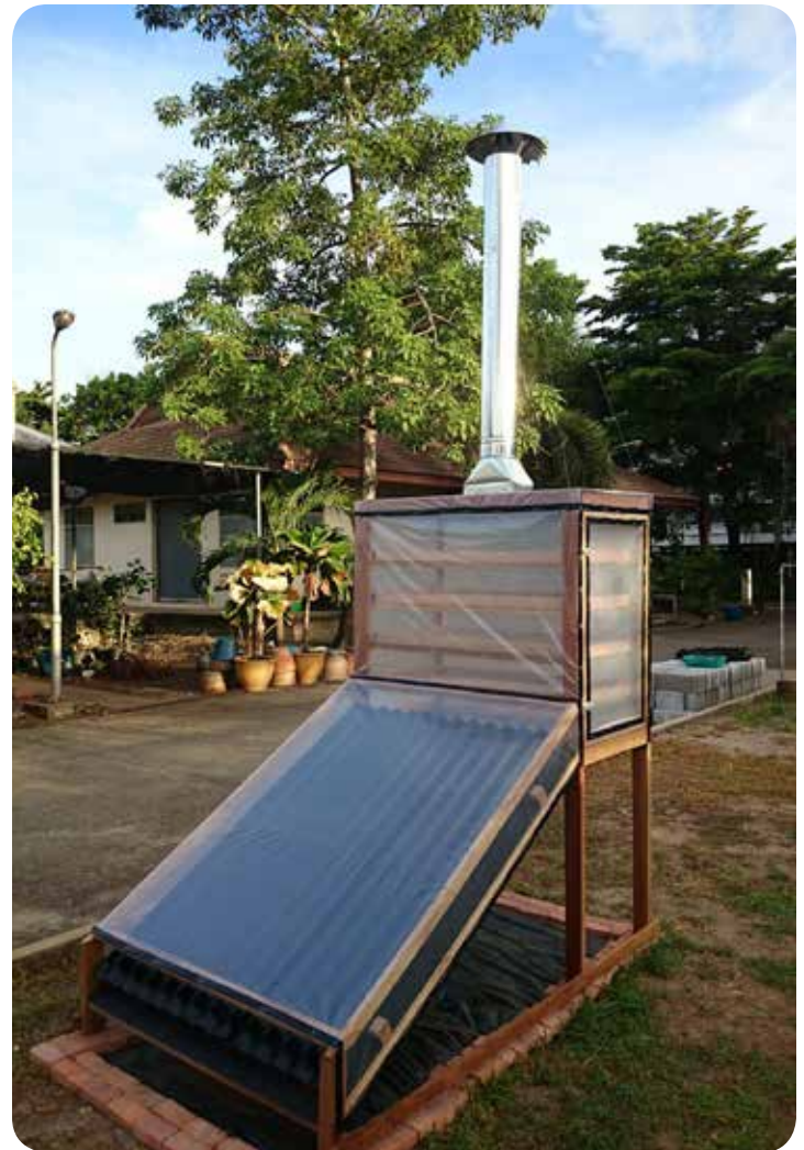
Indirect solar dryer viewed from the front; note chimney for faster air movement and the corrugated black surface in the heating chamber - Photo: Lizanne Wheeler
