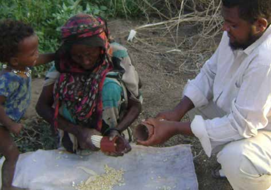
PEF graduate Ibrahim Seid demonstrates a $1 tool that shells 20 kg/hour [bit.ly/2vF9ibd], at the Agricultural Mechanization Research Center in Ethiopia - Photo: Mekbib Heilegebrile Seife - PEF Graduate, Ethiopia, 2012
