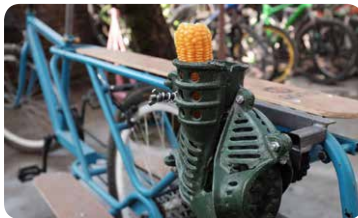
Rotary sheller attached to a PortalBike pedaling set-up in Nepal - Photo: PortalBike
