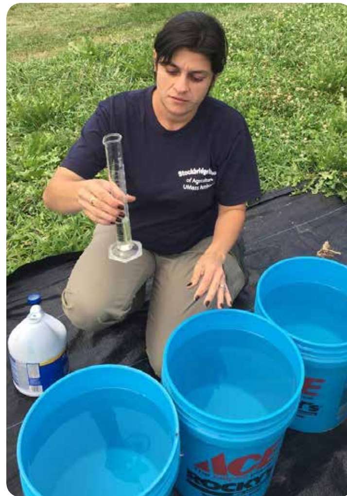
Preparing to use test strips for chlorine wash of cilantro directly in the field, U Mass Amherst - Photo: Zoraia Barros
