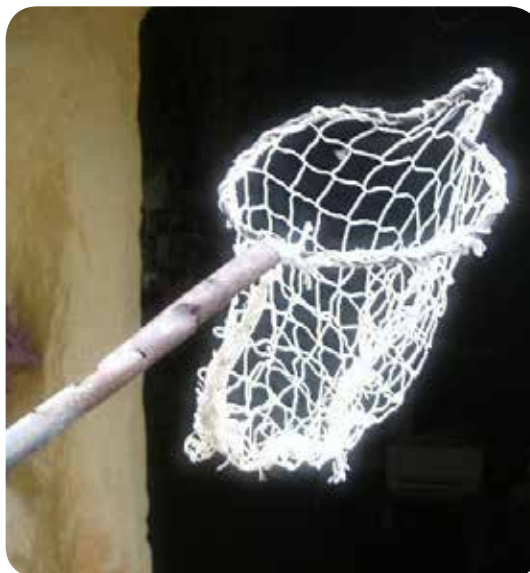
The finger shape on the net's rim guides the fruit into the basket - Photo: John Birdsall
