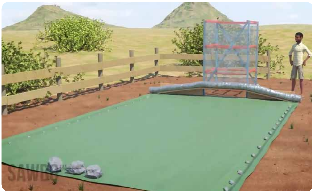
SAWBO-Animations' rendering of a DIY high velocity solar grain dryer. Grains are spread on the ground tarp and the clear plastic is rolled on top. Air flows in through the bottom where the large rocks raise the clear plastic; moist heat flows out through the chimney—Illustration: SAWBO Animations [SAWBO-animations.org]
