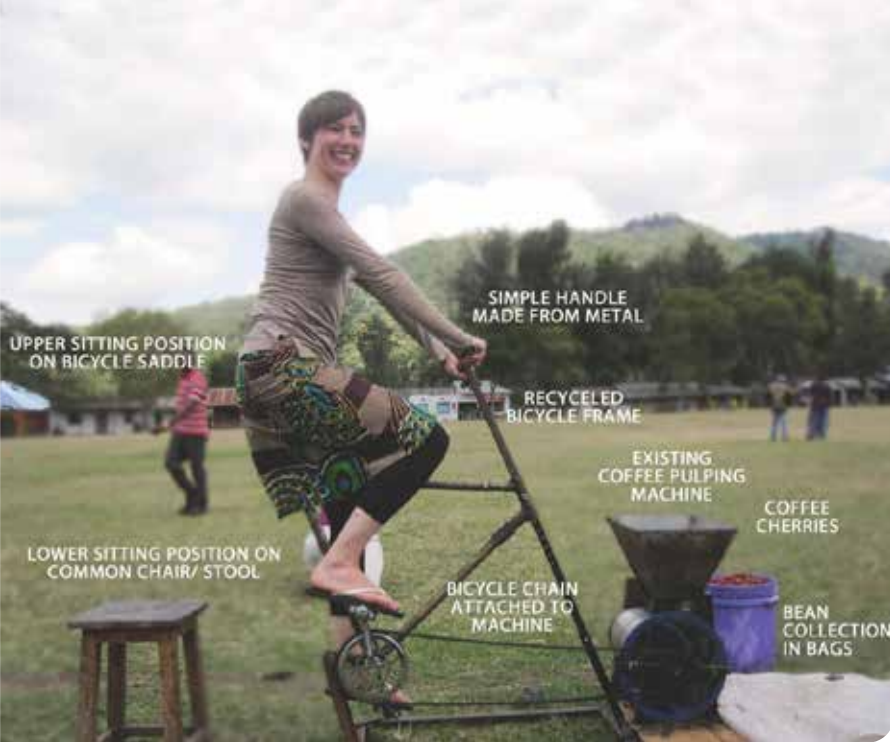
Tanzanian prototype of pedal-powered coffee bean dehuller - Photo: MIT D-Lab (permission requested)
