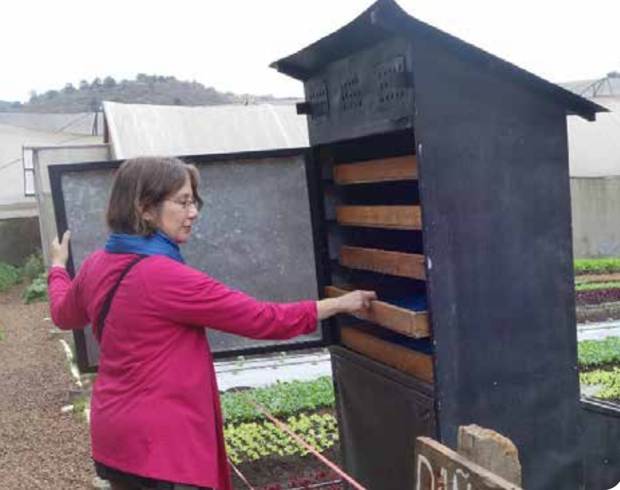
This book's author Betsy Teutsch tests slide-out racks in the drying chamber of Caoba Organic Farm's indirect solar dehydrator, Antigua, Guatemala - Photo: Dina Tanners
