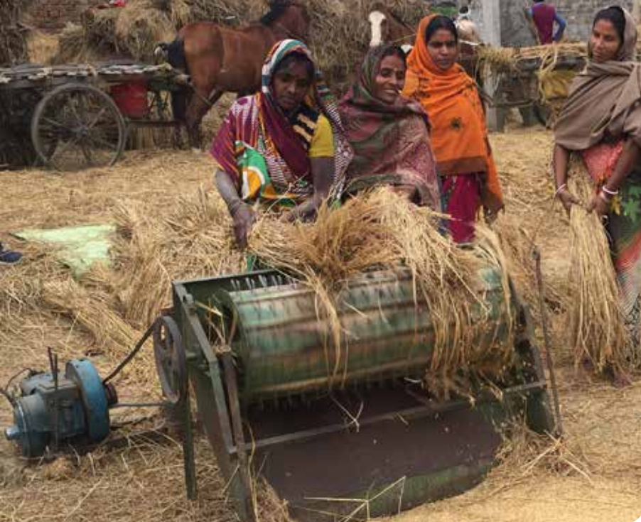
Women during hands-on training using a mechanical thresher learning first-hand how the equipment, which is easy to operate and much less work, can also save time and reduce threshing losses. The chaff flies off and the grain drops into a collection pan at the machine's bottom - Photo: ADM Institute for the Prevention of Postharvest Loss
