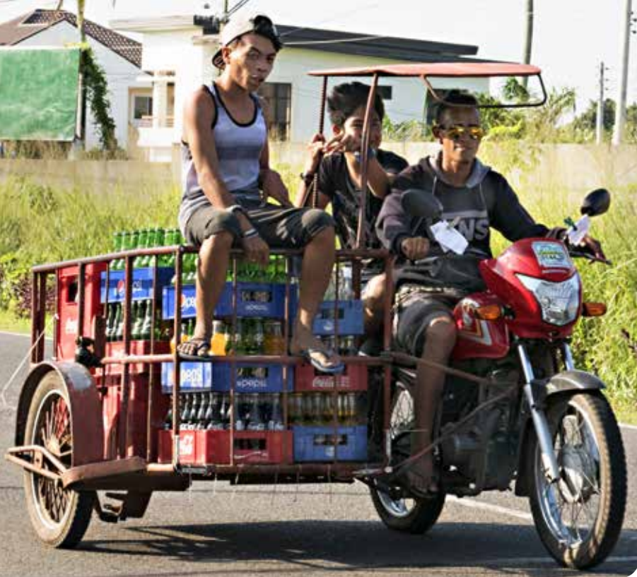
Motorized tricycle delivery vehicle with a mini-sunshade in Silay City, Philippines; such a canopy could be extended to cover the load as well as the driver - Photo: Brian Evans/Flickr
