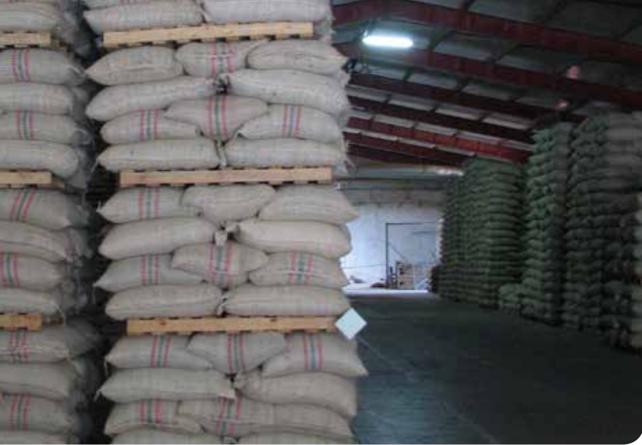
Towers of cross-stacked coffee sacks, reinforced with pallets, in Colombia - Photo: CounterCultureCoffee/Flickr
