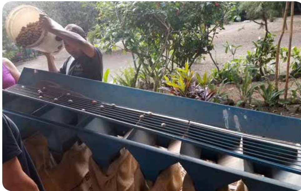
Worker dumps macadamia nuts at the top of the diverging bar sorter at Valhalla in Antigua, Guatemala - Photo: Marni Davis
