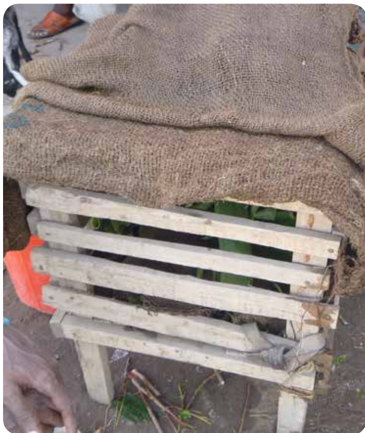
Mini-evaporative cooler for leafy greens in packinghouse, Ethiopia - Photo: Lizanne Wheeler
