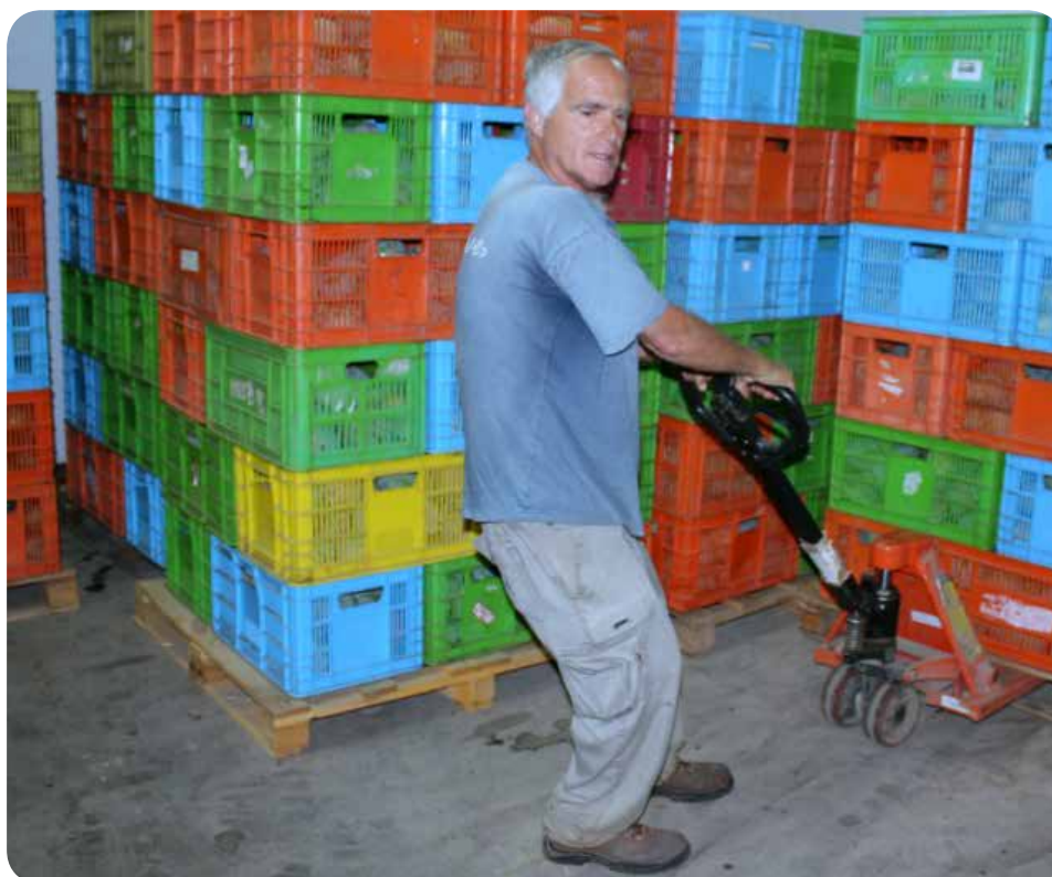
Worker with a pallet jack moving mango in reusable plastic crates at Kibbutz Matsuva, Israel; cross-stacking adds strength to the stacks - Photo: Max Nathans/Flickr
