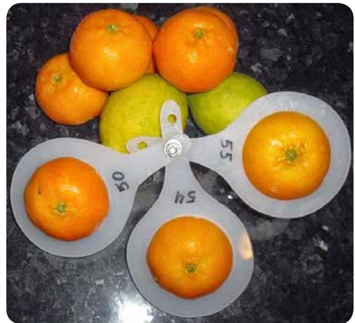
DIY citrus sizing rings designed by El Zeta; instructions are available online [bit.ly/2vFI05W] - Photo: El Zeta
