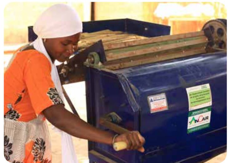
CTI's co-created crank-operated pearl millet thresher/winnowing in Senegal - Photo: CTI
