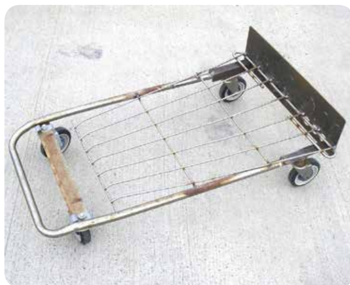
Tim Anderson's hand dolly fashioned from a trashed supermarket cart doubles as a flatbed - Photo: Tim Anderson/Instructables
