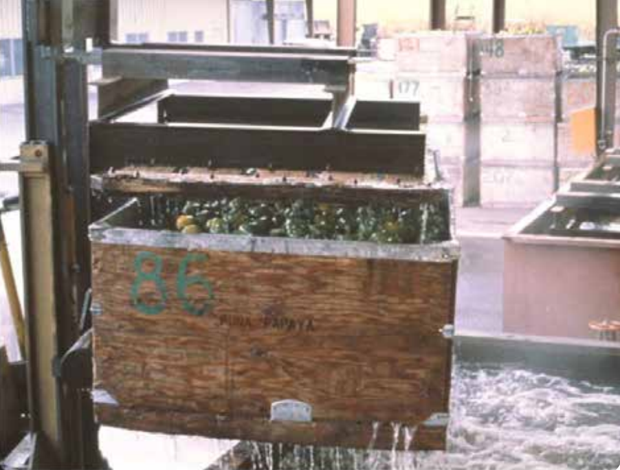
Hot water treatment of papayas - Postharvest Handling of Mango, UC Davis, slideplayer.com/slide/6299318/
