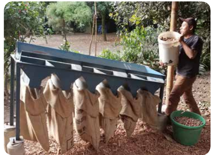
Side view showing collection bags for six sizes of macadamia nuts - Photo: Marni Davis
