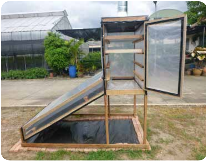
An indirect solar drying unit, Thailand - Photo: Lizanne Wheeler
