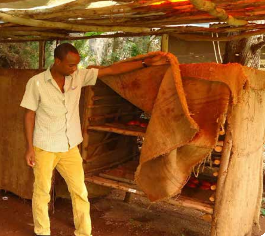
Desert cooler cabinet managed by Esa Abiso, cooling tomatoes in Ethiopia - Photo: Esa Abiso - PEF Graduate, Ethiopia, 2014
