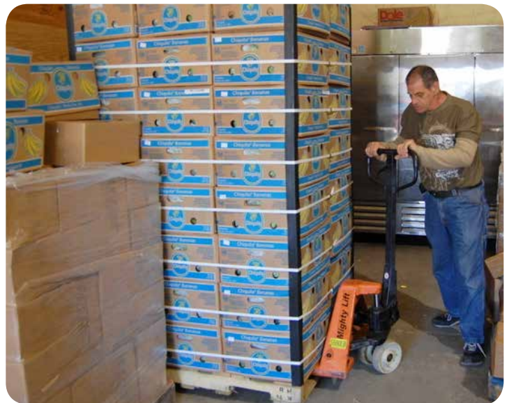
Corner reinforcements on a pallet of bananas at the St. Bernard's Parish Community Center, New Orleans, LA - Photo: CC of St. Bernards
