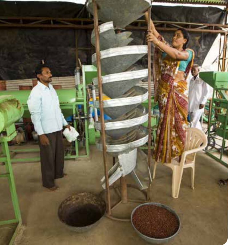
This lentil separator or “dal mill” separates lentils from pebbles and debris; it processes as many lentils in five minutes as would normally take a woman all day - Photo: IFAD/Susan Beccio
