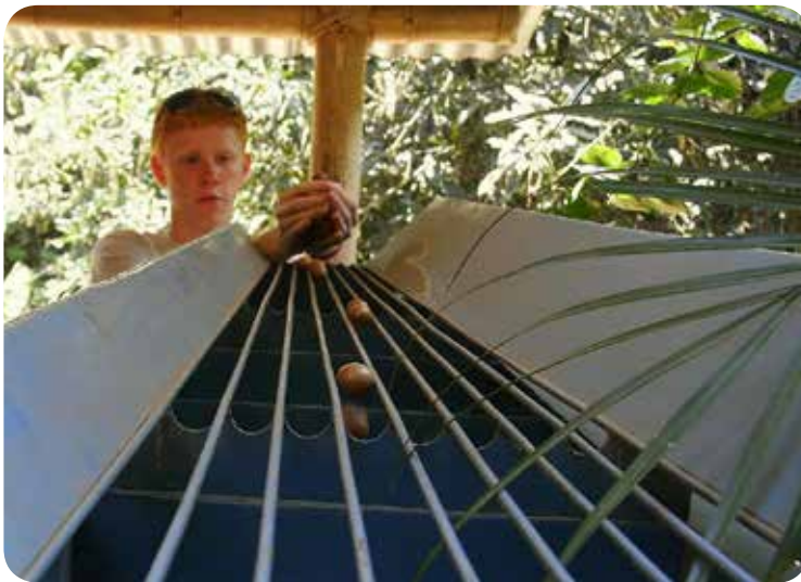
Ben Miller rolling macadamia nuts down the diverging bar sizer – Photo: Nathan Shelburne
