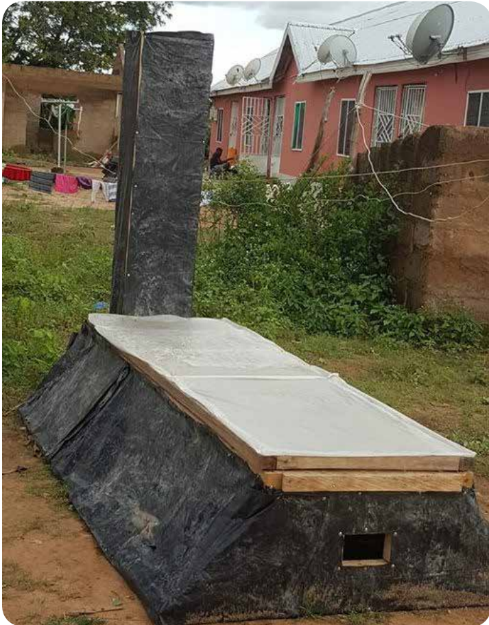
Postharvest Educator Kodimah Issifu's "simple mixed mode solar drier [bit.ly/2pYWY2D] for preservation of my veggies in glut. Thanks to Emmanuel Ayua for the design." Issifu estimates it cost around $40 in materials. The black trapezoid base provides more solarization surface for heat collection, to warm the inner air flow through the chamber and up through the stack - Photo: Kodimah Issifu - PEF Graduate, Ghana, 2014 - posted on Facebook
