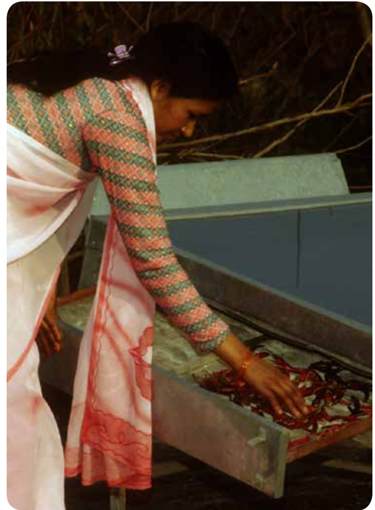
A group member of the FAO TeleFood project dries chilies in a stainless-steel solar dryer with a glass cover and slide-out tray in Nepal -©FAO/ Diana Giampiero
