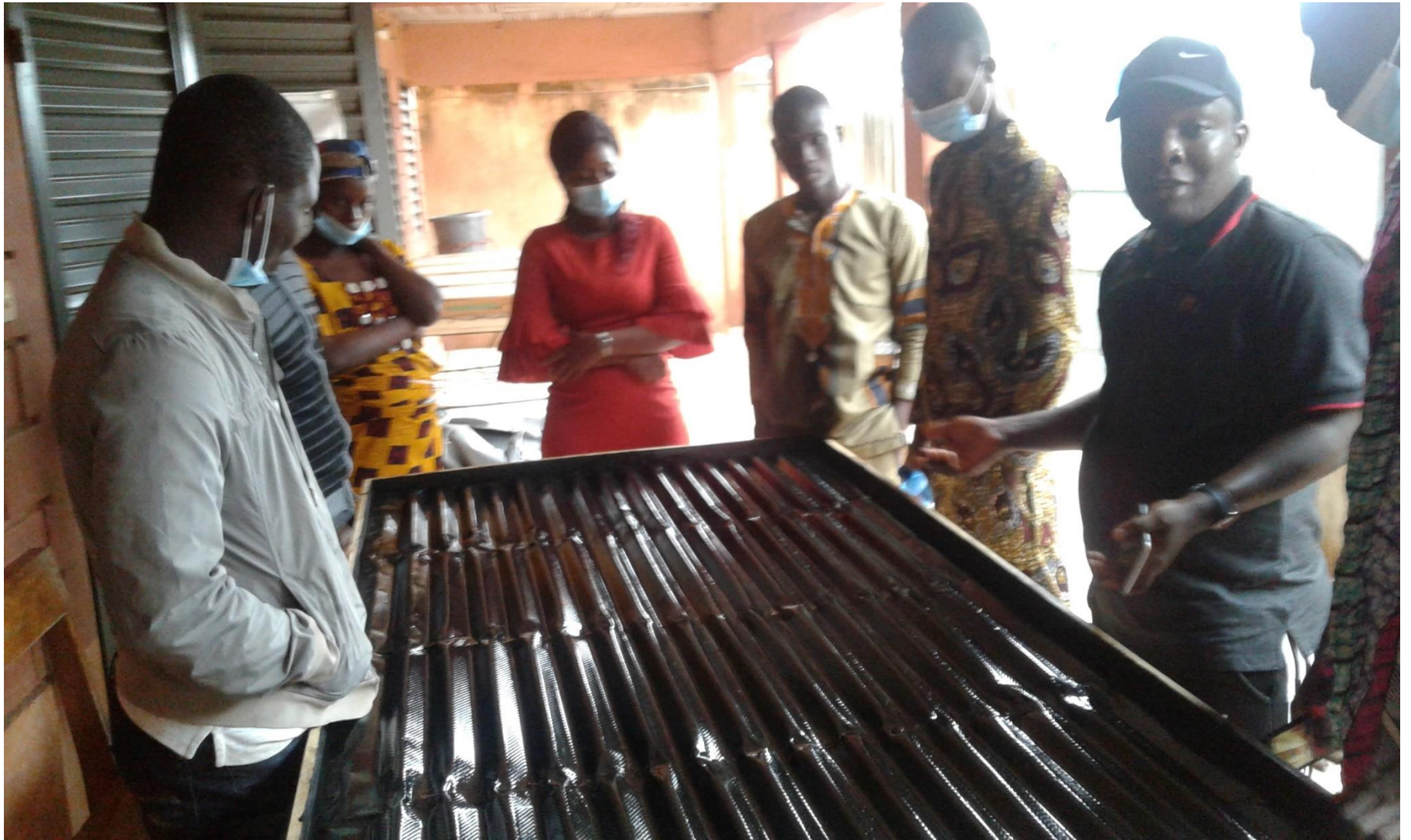
Figure 1. Presentation of solar radiation black absorption surface of a solar dryer, how it works and how to construct.
