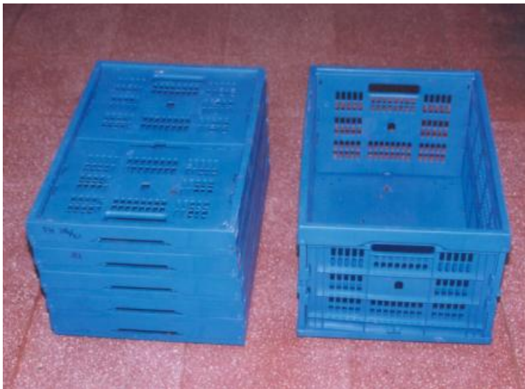
Figure 17: Collapsible RPCs in use in Sri Lanka (photo is showing how the volume of 5 folded crates = 1 open crate). Visit TranPak Inc's website to watch a short video of collapsible RPCs: http://www.youtube.com/watch?v=UI7tRlq_-BY
