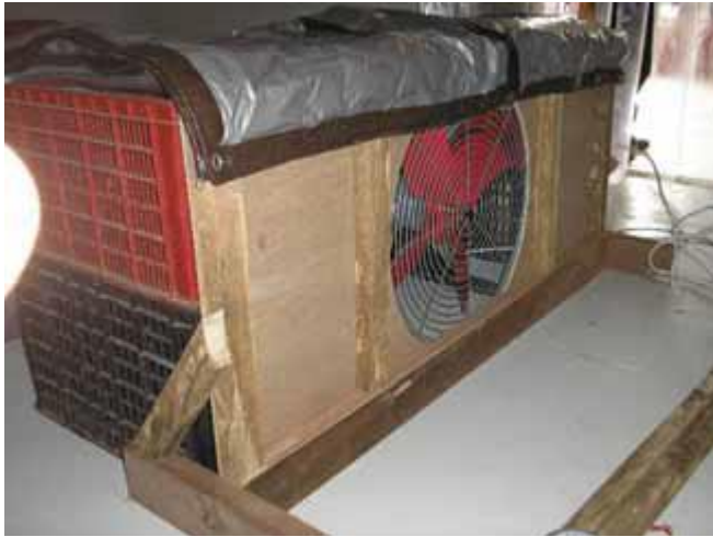
Figure 23: Use of RPCs during forced air pre-cooling in Bali, Indonesia (Photo credit: Lisa Kitinoja, 2007)
