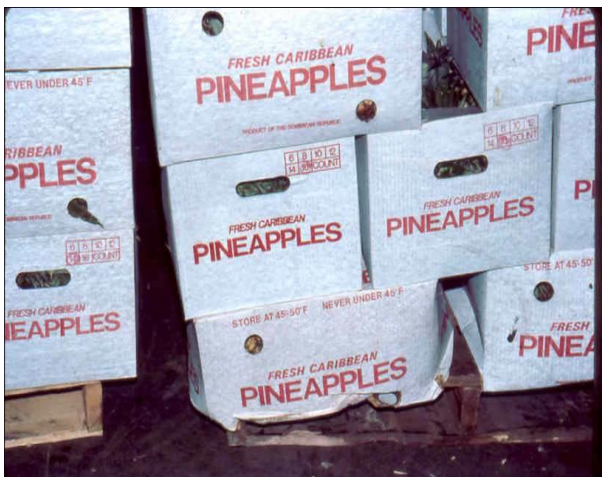
Figure 6: Low quality fiberboard cartons of pineapples collapse during high humidity cool storage (McGregor, 1987)
