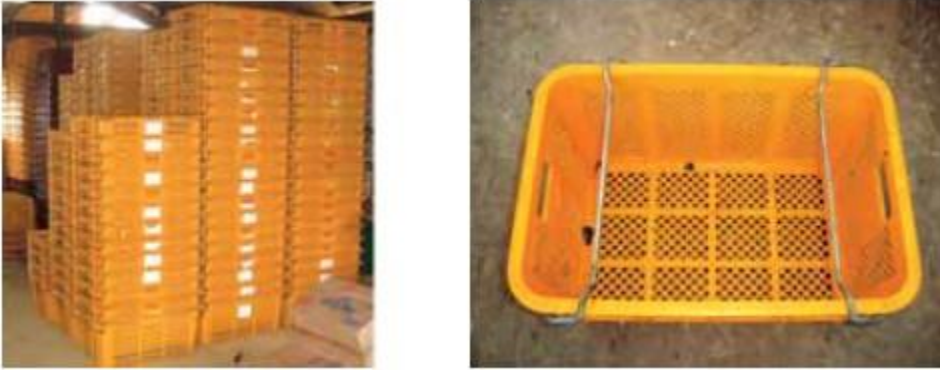
Figure 15: RPCs nested for return transport (Rupasas and Rolle, 2009)
