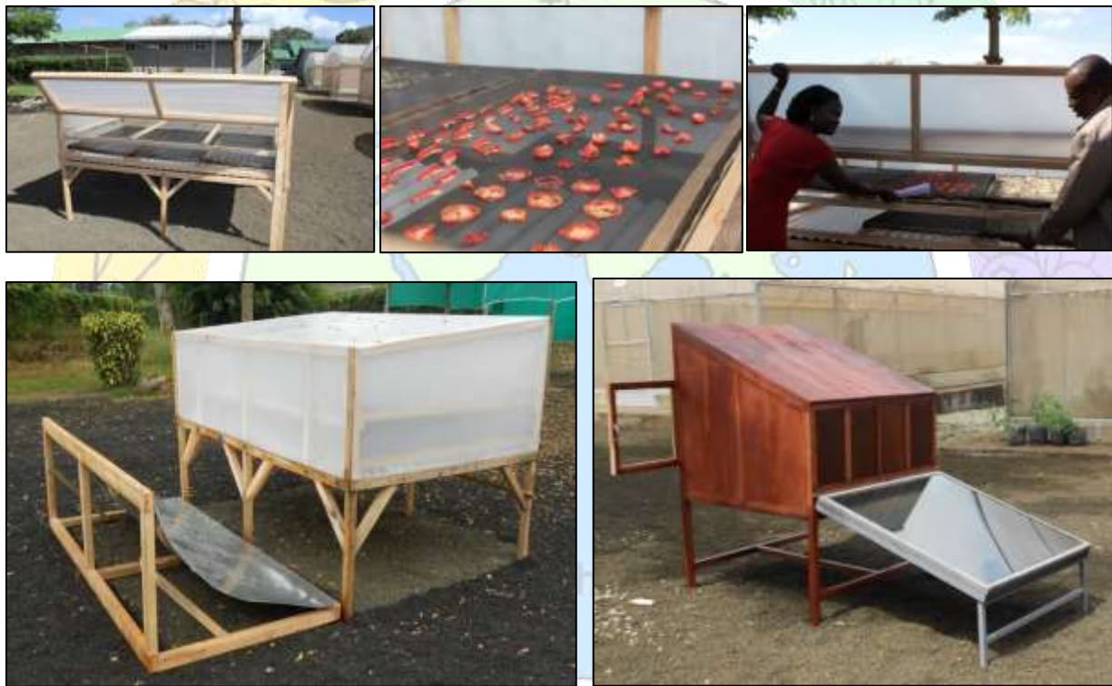
Reflector added to a simple direct dryer, and improved indirect cabinet dryer with solar collector (still needs to have a chimney added)
