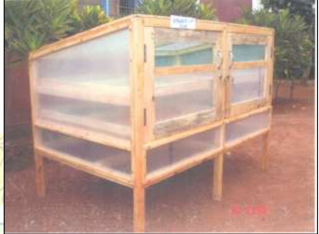
Photo of a solar dryers used for training and small-scale produce drying businesses in Tanzania
