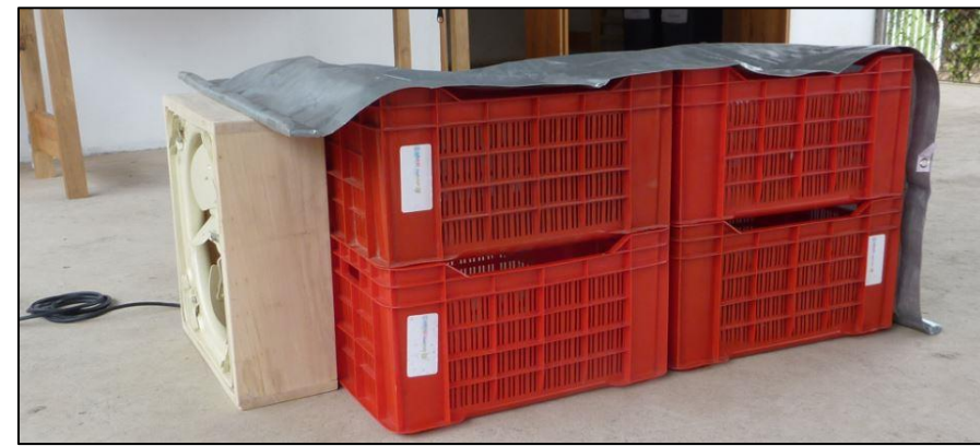
Portable forced air cooling tunnel
