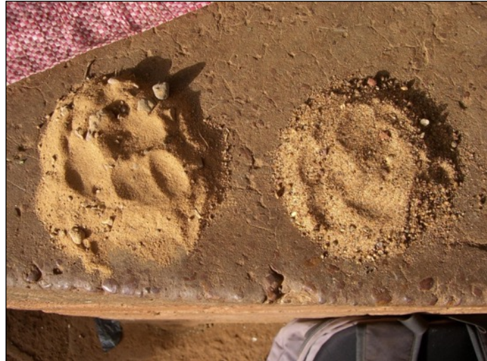
The sand on the left contains too many tiny clay particles.
