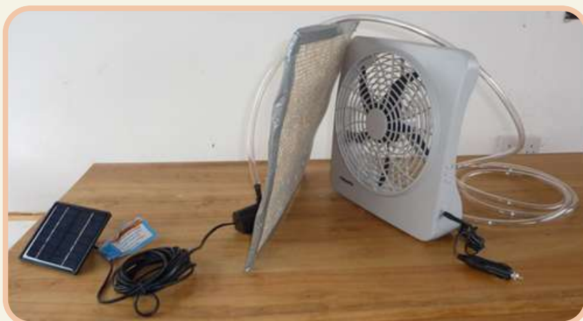
A simple, portable evaporative cooling demonstration
