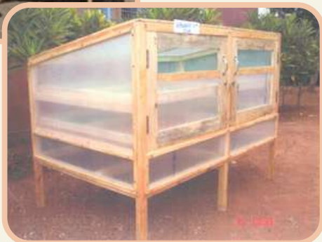
Photo of a solar dryer used for training and small-scale produce drying businesses in Tanzania
